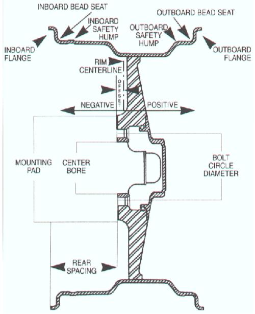
**Bolt pattern** or **lug pattern** or **bolt circle** is determined by the number of bolt holes and the bolt circle diameter.
