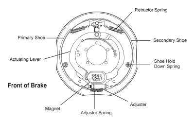
When the electrical current is fed into the system by the controller, it flows through the electromagnets in the brakes. The high capacity electromagnets are energized and are attracted to the rotating armature surface of the drums which moves the actuating levers in the direction that the drums are turning.
