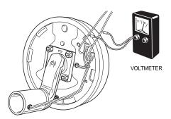
The threshold voltage of a controller is the voltage applied to the brakes when the controller first turns on. Lower threshold voltage will provide for smoother braking. If the threshold voltage is too high, the brakes may feel grabby and harsh.
