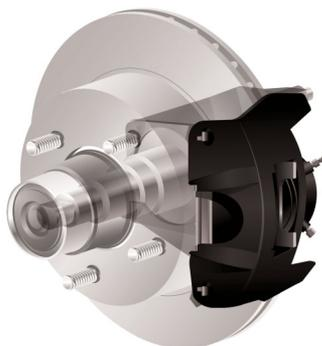
Disc brake effectiveness is the same going either in a forward or reverse direction. All Dexter disc brakes should be actuated with a braking system that is capable of providing a maximum hydraulic pressure of 1,600 psi.
